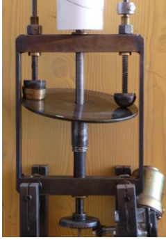
Figure 1. The swash plate mechanism
